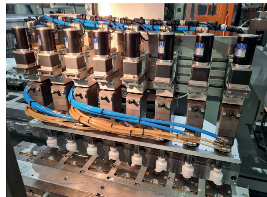
Detail of Mod. PB15ED-800 – 8+8 cavities for the production of yogurt bottles.
